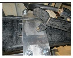
Place convoluted tubing over lines where they cross the mounting bracket to protect the lines. Secure in position using silicon inside the tubing or similar. Move lines away from mounts to ensure they do not rub.
